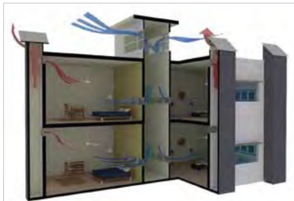
Figure 5 Downdraft cooling system
