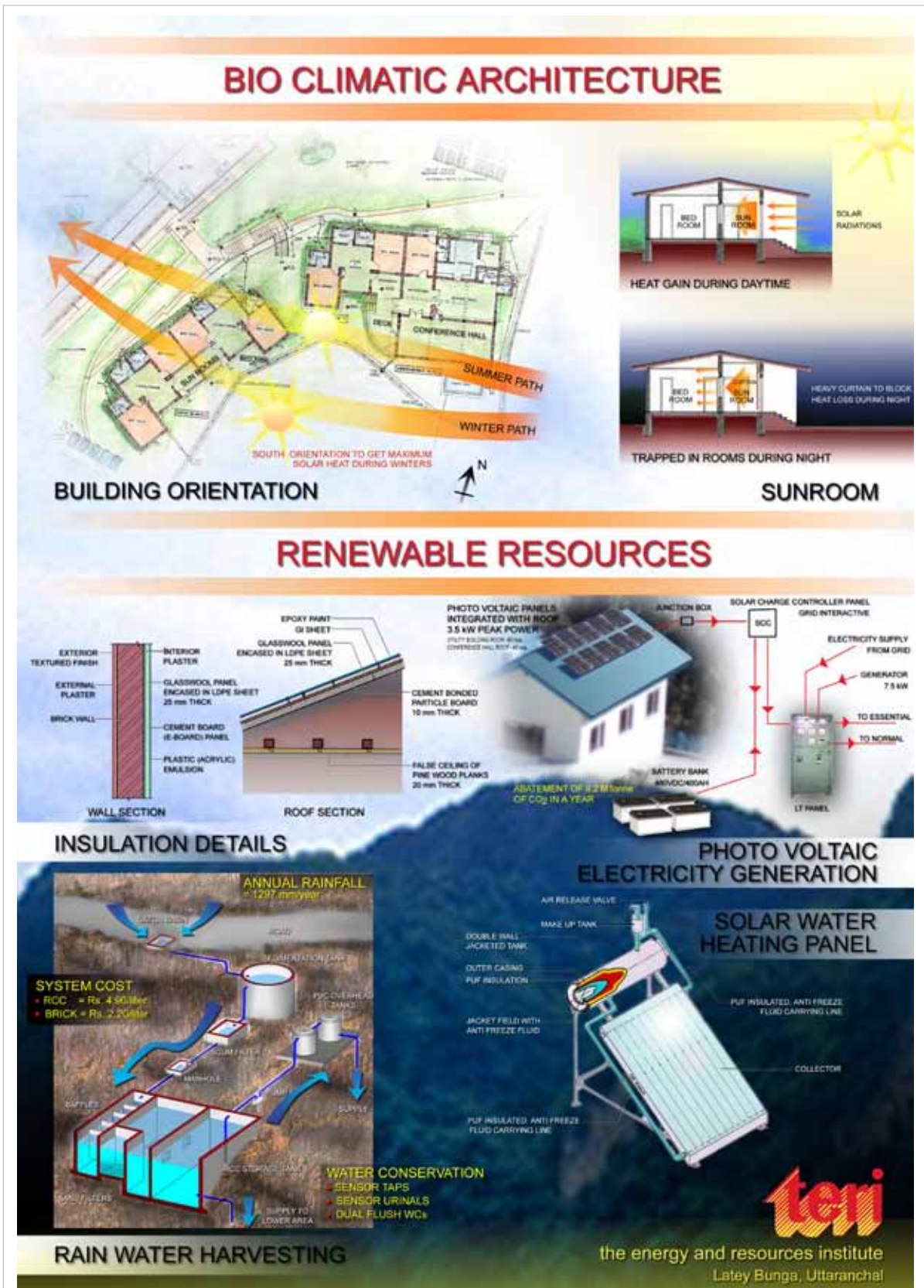
Figure 6 Low energy strategies in TERI - Mukteshwar building
